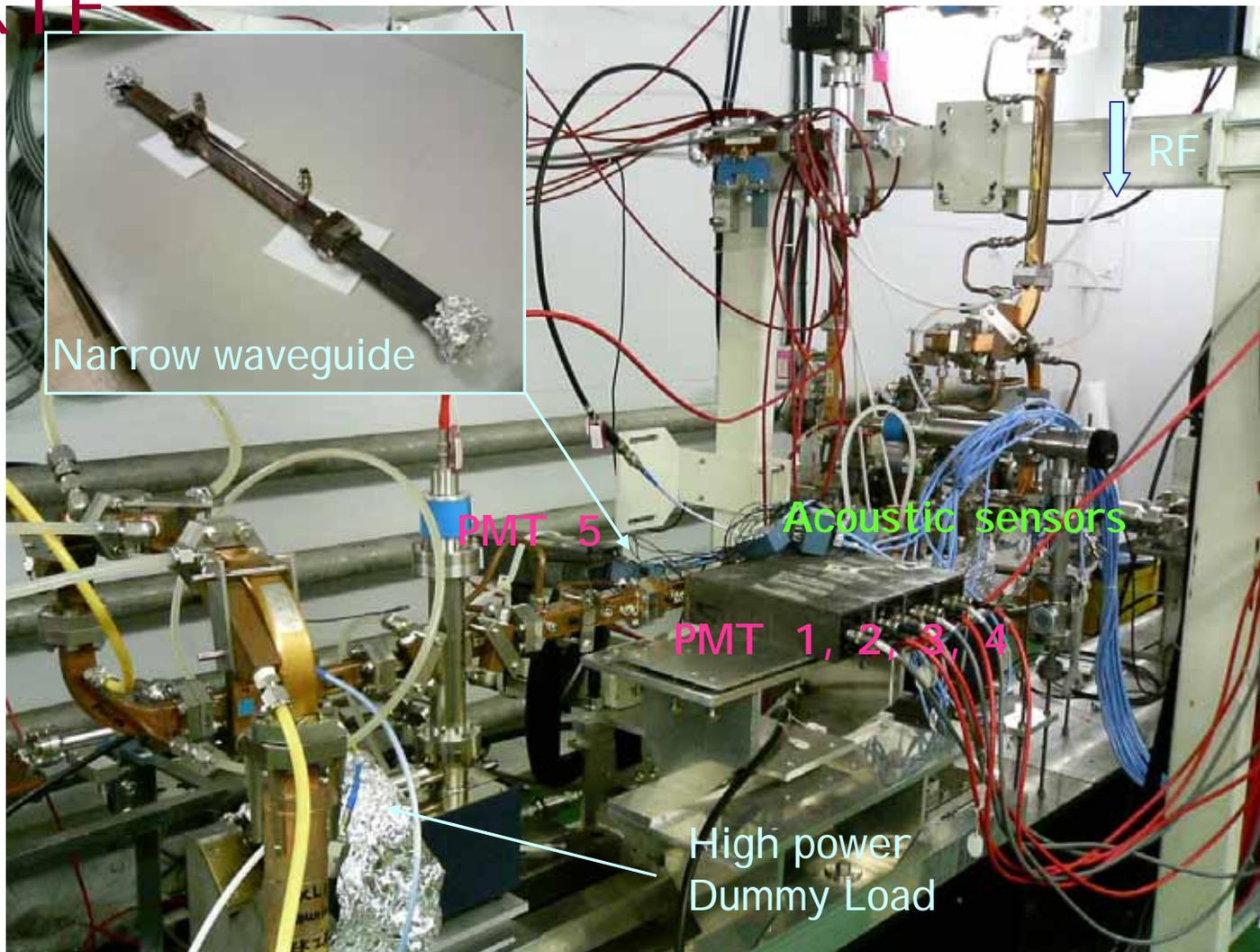
➤ The first high-power test of copper(Cu002) was done at XTF (previous X-band Test Facility at KEK).
